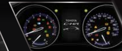
OPTITRON COMBINATION METER WITH 4.2" TFT COLOR MID
